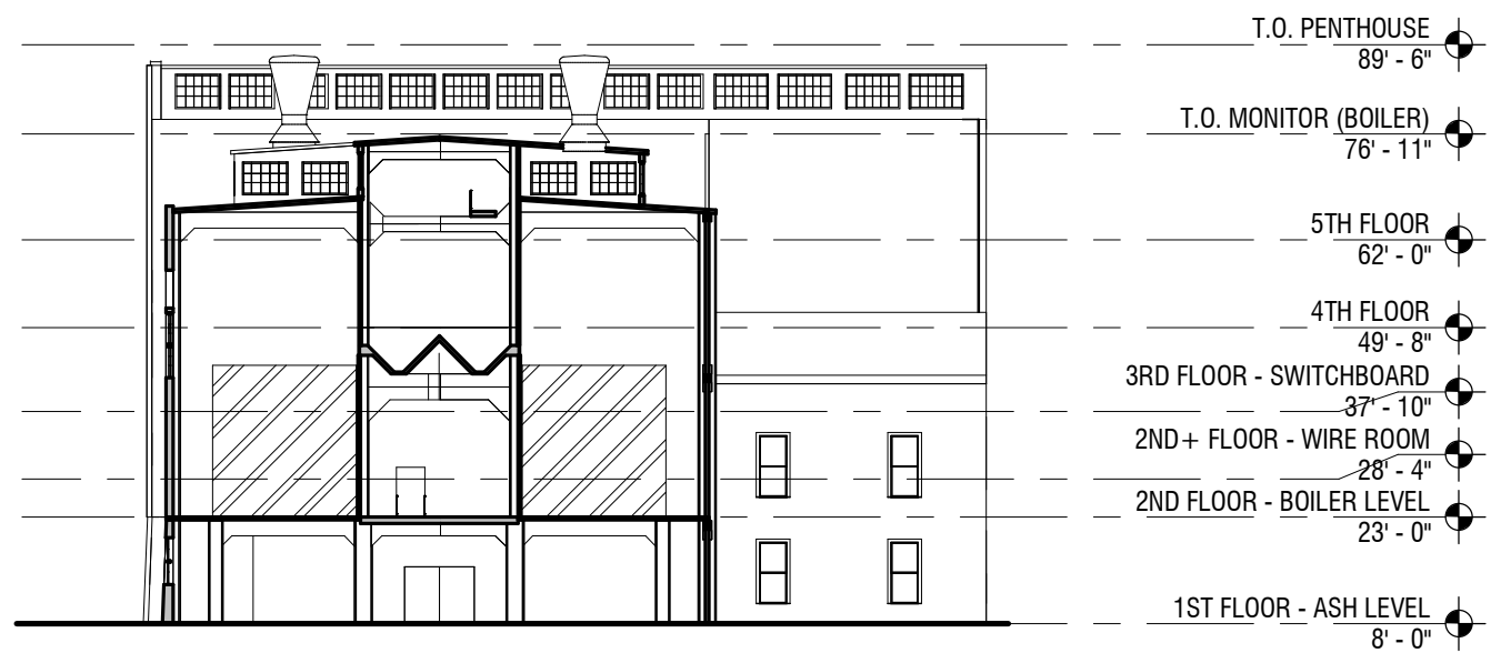
2 (E) SECTION THROUGH BOILER ROOM 1" = 30'-0"
